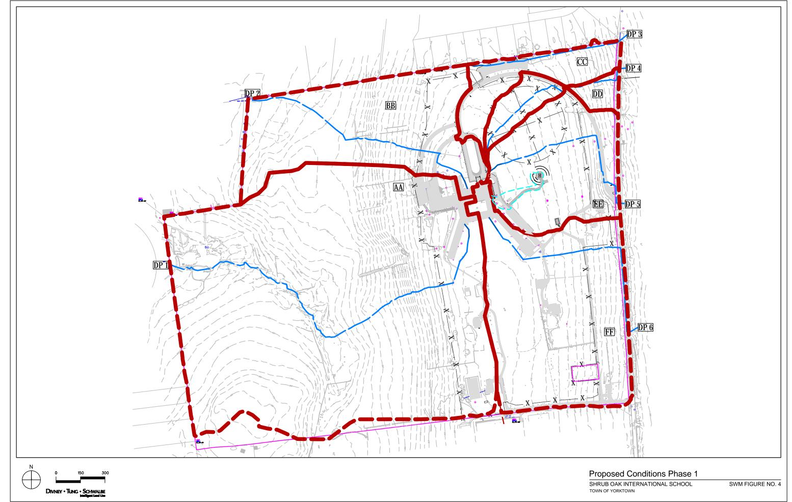
Because of existing infrastructure and in order to minimize the limit of disturbance, 100% of the Water Quality Volume (WQv) is not feasible. The NYSDEC Design Manual allows for the specific reduction factor (S) of 0.3 to be applied within hydrologic soil group (HSG) C.
